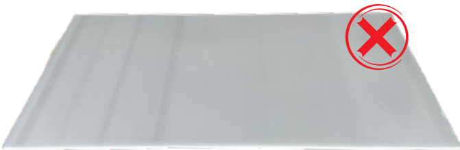
DARK BANDS VISIBLE TO THE NAKED EYE AT A DISTANCE OF 1 METRE
